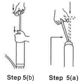
**Step 6: Unscrew gun head 1-3 turns and pump the lever handle around 6-8 times until grease comes out. This releases air pockets from barrel and makes it easy to pump the grease.**
