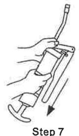
**Step 7: Screw the gun head tightly and ready for priming.**
